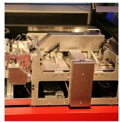
ments and empty envelopes during the inserting process. With these two options and the standard document monitoring system, the machine is able to divert faulty documents or envelopes preventively.
